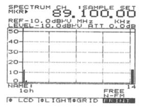
Grid 1: Horizontal and Vertical grid lines are displayed
