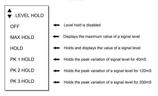
**A LEVEL HOLD** mode may be operated at all times while the 3201 is running. Prior to scanning in a **HOLD** mode set all signal levels amplitudes to their minimum value or 0dB.
